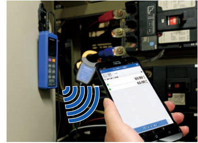
Measurement results will be sent to the tablet wirelessly and displayed.
