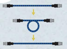
The cable was wrapped  $360^{\circ}$  around  $\phi 60$ mm mandrel. \*Guaranteed value within ±5.7°at 26.5GHz (In shipping value)
