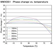
The cable was measured in chamber every 20  $^{\circ}\!\text{C}$  from -30 to 90 °C, 1 hour after the temperature changed. Figure shows the excellent phase stability over the temperature changes.
